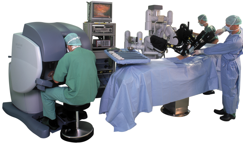
Fig. 1.18: Replicating the surgeon's hand motion with a robotic interface mounted to the patient couch (da Vinci Surgical System, Intuitive Surgical, Inc.)
