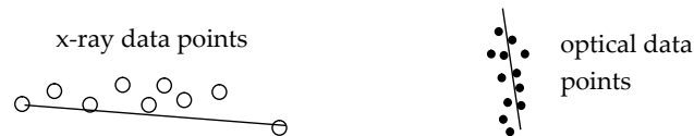
Fig. 7.4: Data points from optical tracking and x-ray imaging. Both types of sensor data points have time stamps. This allows for establishing the correspondences between the data points.
